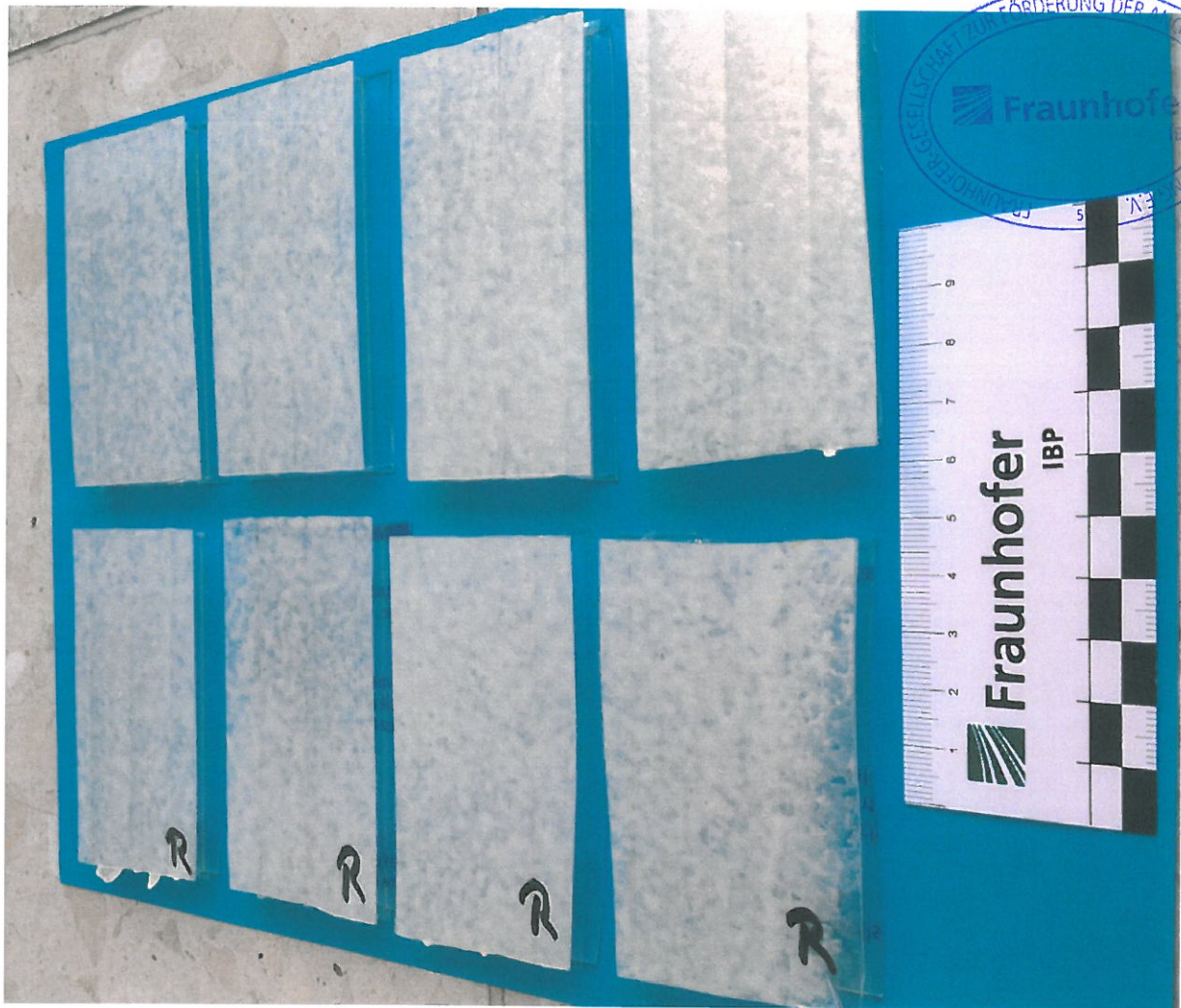
Figure 2: Selection of samples in new condition (marked with "R"), and after weathering, as seen from a different viewing angle.
