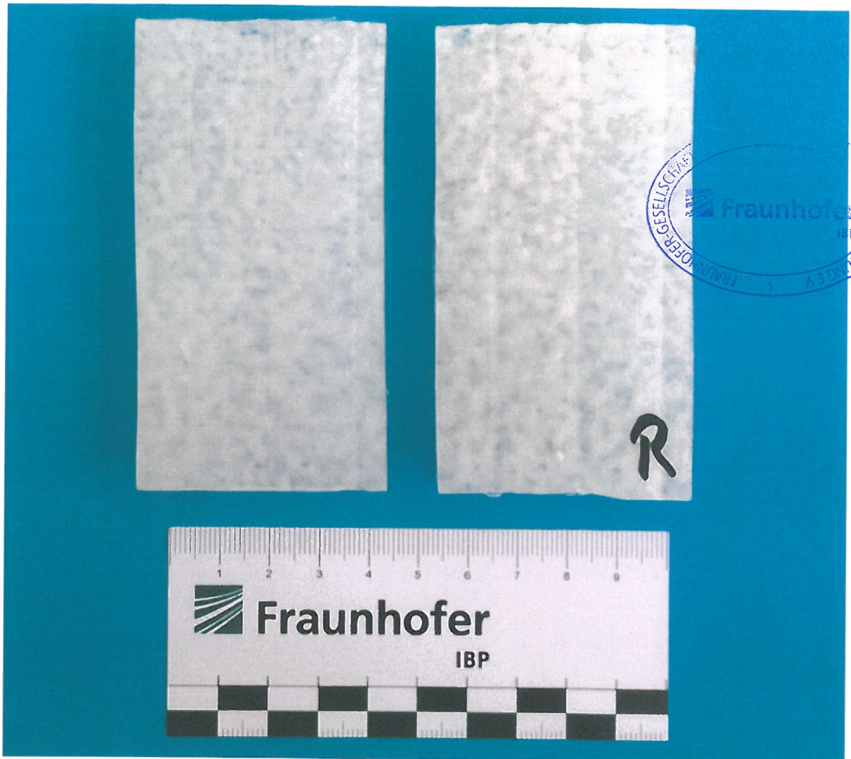
Figure 3: Close-up of two samples. Left side after weathering, right side in new condition (marked with "R").
